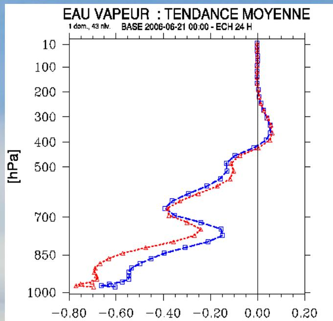
Water vapour tendency for two entrainment rates for 21.06.2006, 00+24 h:
