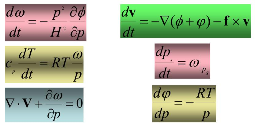
**v** –horizontal wind vector, **\omega** – vertical (omega-)velocity, *H***=***RT/g* – scale height, **\phi** – non-hydrostatic geopotential, **\phi** – hydrostatic geopotential, *R*, *C*<sub>*p*</sub> – gas constants, *p* – pressure, *p*<sub>*s*</sub> - surface pressure
