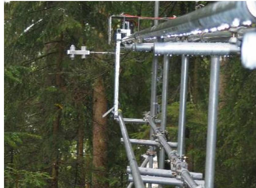
Moving net-radiometer on a 10 meter long rack
