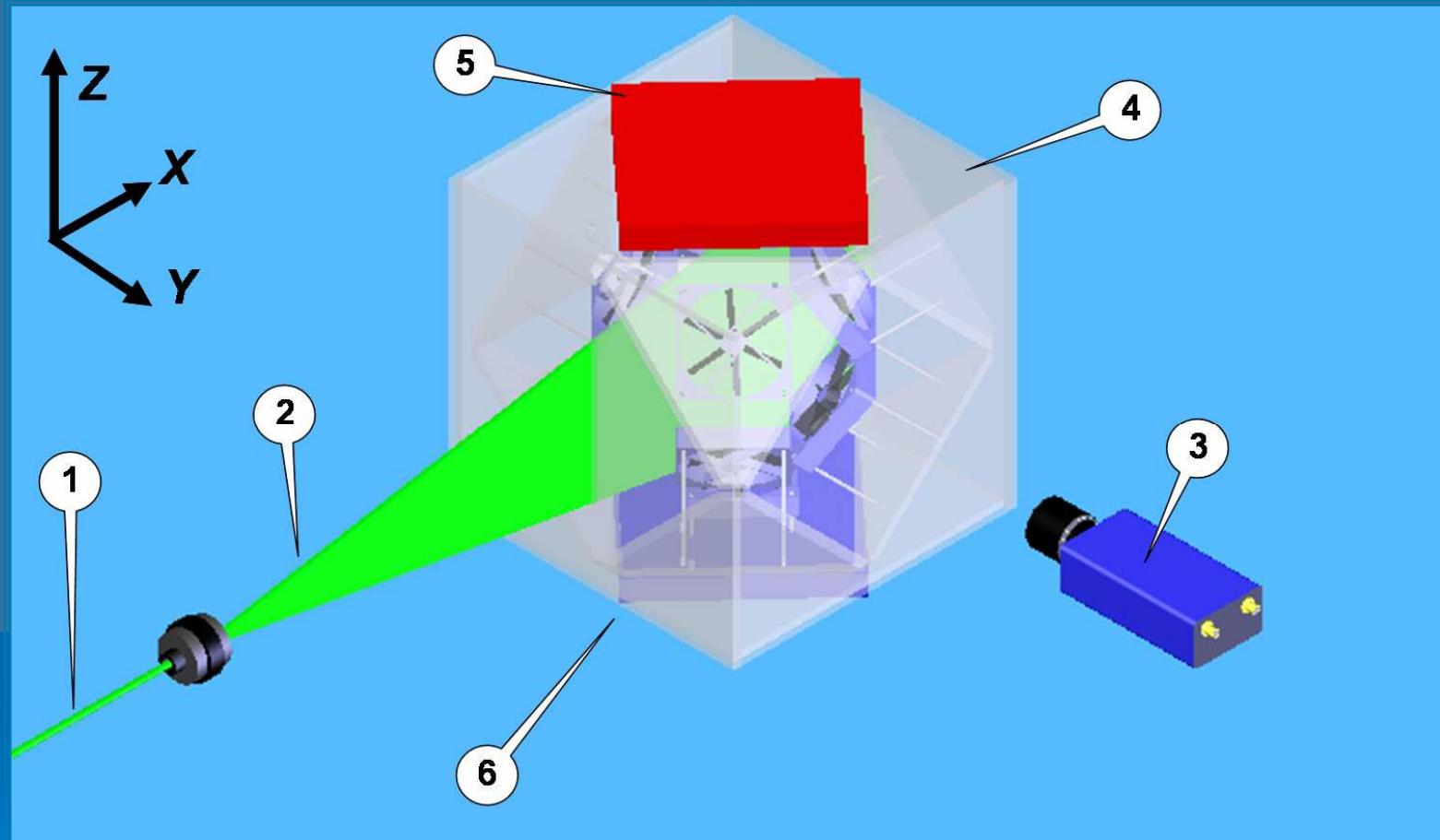
1- laser beam, 2- light sheet, 3- CCD camera, 4- test section,
