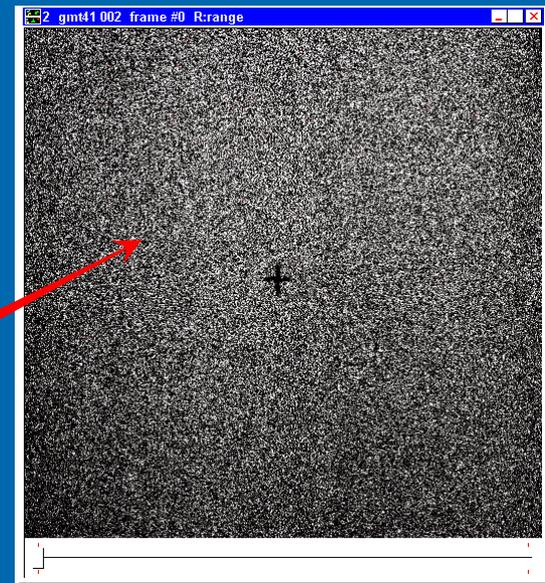
Raw image of the incense smoke tracer particles in oscillating grids turbulence
