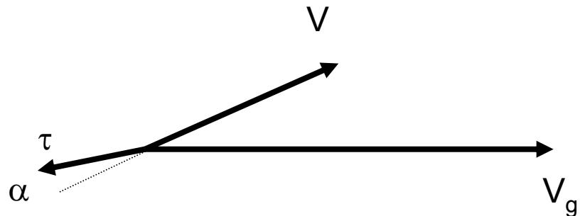
**The turning angle  $\alpha$  depends on the bulk Richardson number, and varies between 0 for unstable or neutral stratification and  $\pi/4$  for very stable stratification**
