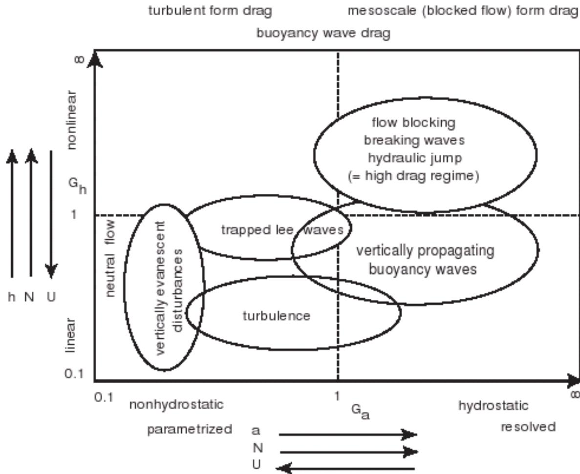
**Orographic flow characterized by non-dimensional height ( $G_h$ ) and width ( $G_a$ ) of the obstacle.** From Rontu, 2007 (pers. comm.)
