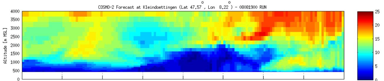
**COSMO-2 WS assimilation cycle for Kleindoettingen using CWINDE profilers**
