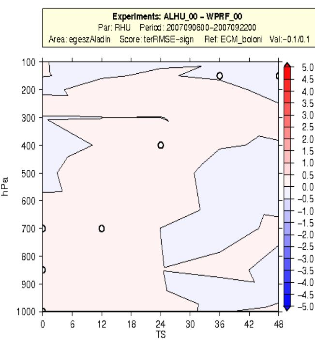
Vertical cross section of RMSE differences as function of forecast range. Red indicates improvements
