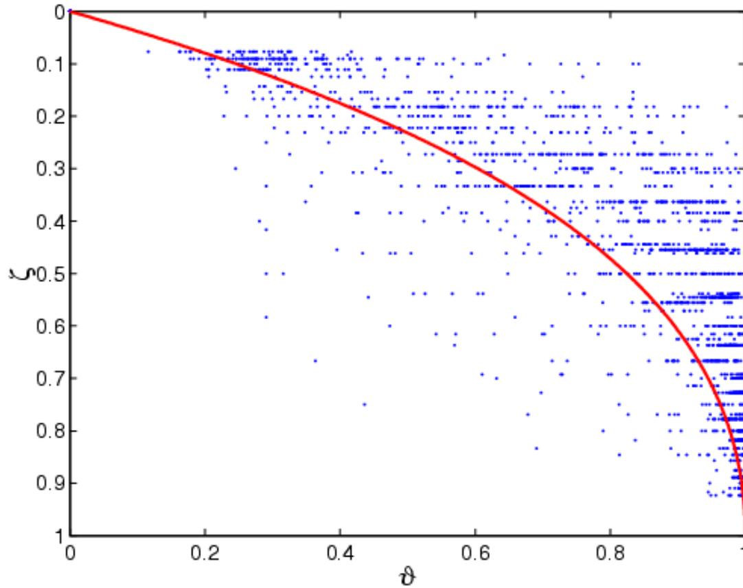
Dimensionless temperature profile in the lake thermocline. Points show data from measurements in Trout Bog (depth=7.7 m). Curves show a polynomial approximation (Kirillin 2002).
