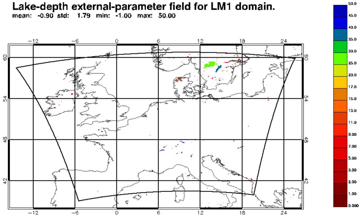
Lake depths for the LM1 numerical domain of the NWP model COSMO. The field is developed (Natalia Schneider) using various data sets. Each lake is characterised by its mean depth.
