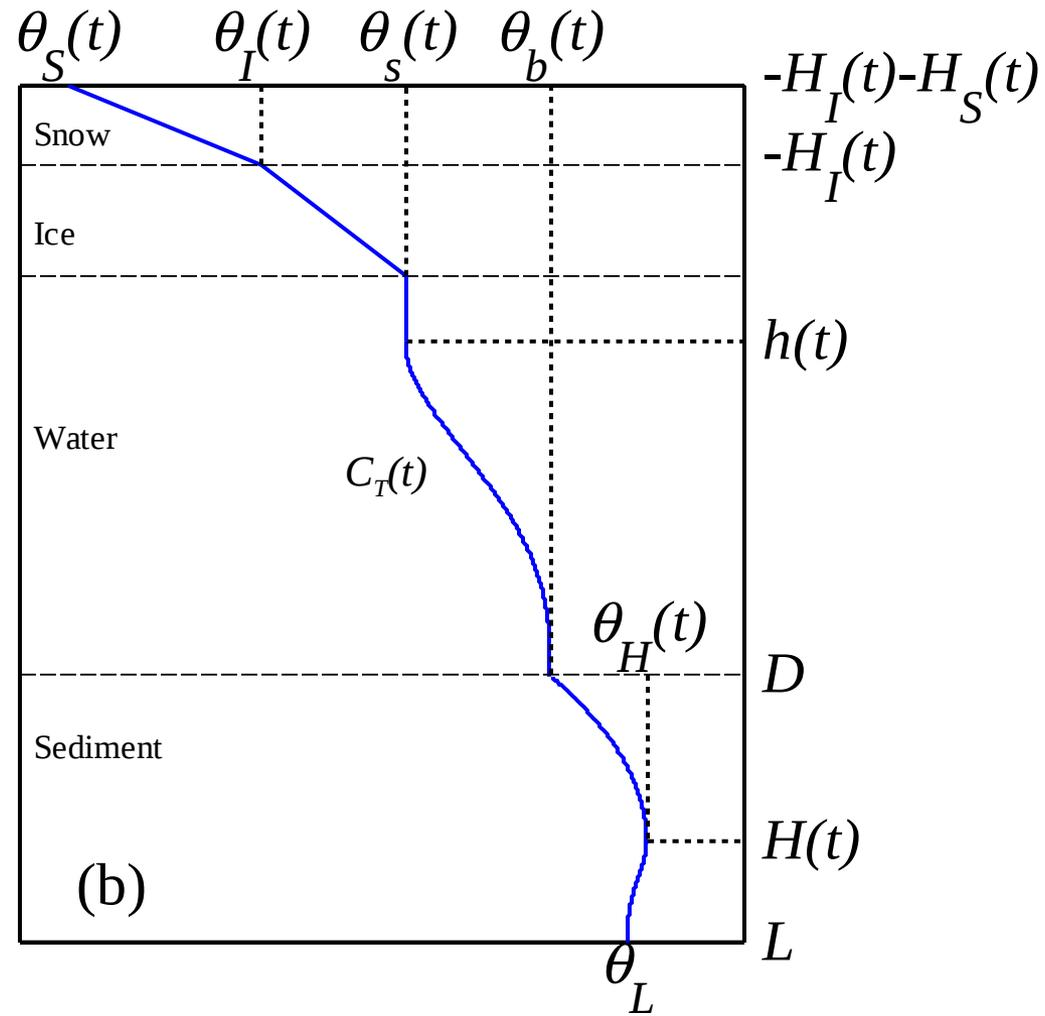
(b) In winter, four additional variables are computed, namely, the temperature  $\theta_S(t)$  at the air-snow interface, the temperature  $\theta_I(t)$  at the snow-ice interface, the snow thickness  $H_S(t)$ , and the ice thickness  $H_I(t)$ .
