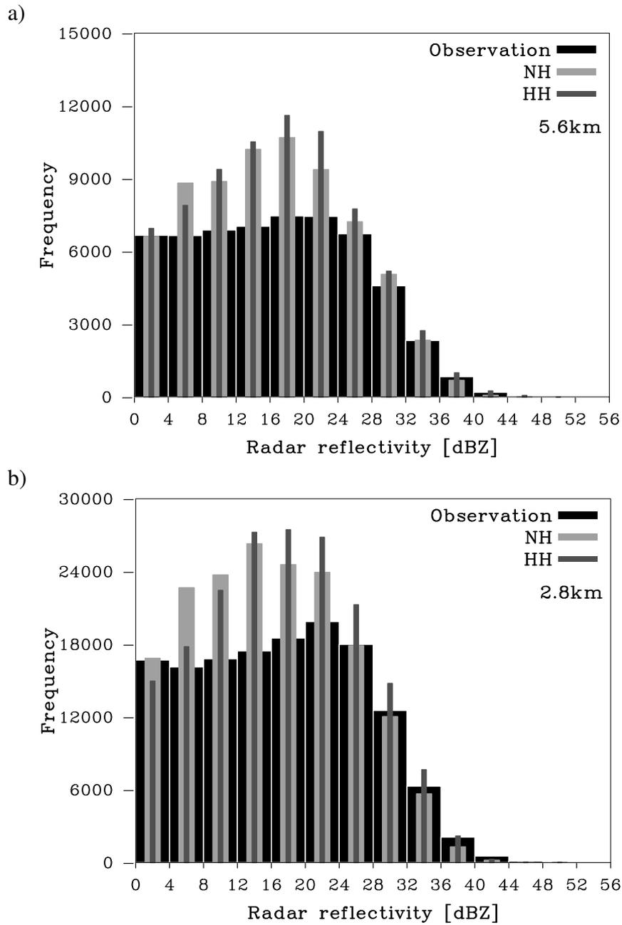
Figure 4: Frequency distributions of radar reflectivity [dBZ] produced by 54 hour simulations starting from 12 UTC 27 July 2004. Grid length is a) 5.6 km and b) 2.8 km. NH- and HH-experiments are represented with light gray and dark gray bars, respectively. Black bars represent dBZ-observations. The elevation of radar antenna is  $0.4^\circ$ . In this case reflectivity values below 0 dBZ are not meteorologically important and therefore those are omitted.
