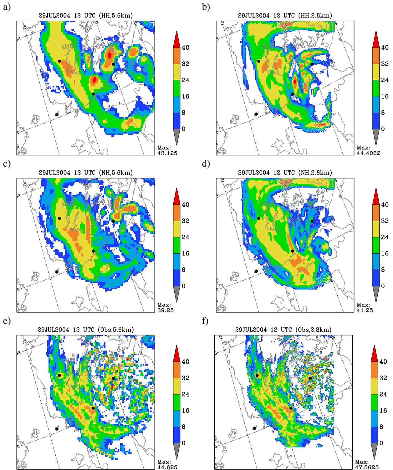
Figure 3: Composite of radar reflectivity [dBZ] fields after 48 hour simulation valid at 12 UTC 29 July 2004. a) HH, 5.6 km, b) HH, 2.8 km, c) NH, 5.6 km, d) NH, 2.8 km, e) radar observation, 5.6 km and f) radar observation, 2.8 km. The locations of the radars are marked with black dots.
